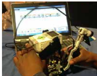
Robotics activities allow learners to build and program their robot using a block-based (BB) programming EV3 interface
